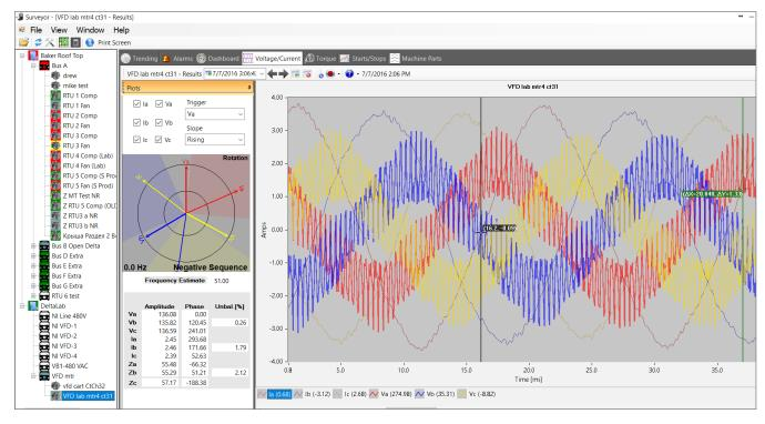
A time waveform plot of a VFD-driven motor, showing voltage and current, with a phasor diagram.
