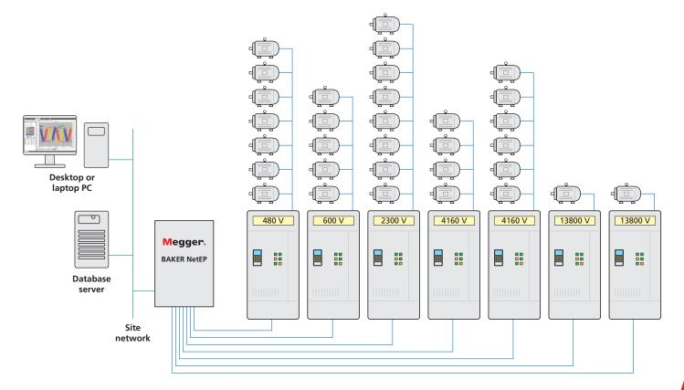
A diagram showing an example of a NetEP installation. The NetEP can monitor up to seven voltage buses, with up to 32 motors in total.
